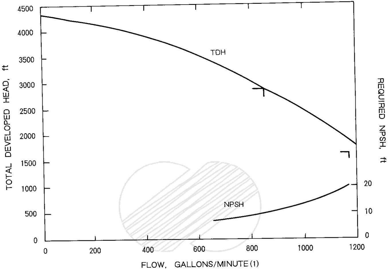
Note 1 : FLOW INCLUDES 85 GPM (322 L/MIN) BYPASS FLOW
